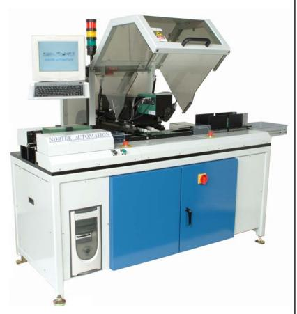
Nortek's SOL850 is the ideal circuit board marking solution, complete with built in de-stacker and re-stacker. By combining board handling with an innovative positioning system the SOL850 provides the highest throughput in the industry. Direct marking eliminates the recurring consumables cost of labels and ink solutions. The laser's durable marks withstand the latest high temperature processes. High resolution, machine-readable codes pack more information in less board space.
